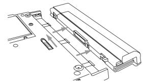
Figure 2-4. Removing the Battery
